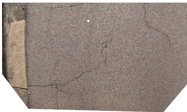
Figure 41. Hugin Output after Omitting Calculate FOV, Calculate Optimum Size, and Fit Crop to Images Steps
