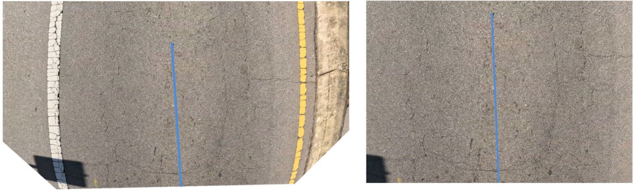
Figure 9. Distortion-Corrected Image (Left: After the First Cropping; Right: After the Second Cropping)
